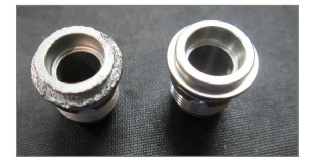
Stainless steel or aluminum parts corrode easily with blood
